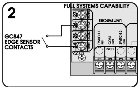
O With full systems capability control boards, the edge sensor is connected to terminals 24 and 26 as shown at left in figure 2.
